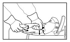
• Release the trigger switch (1) and auxiliary switch (3).
